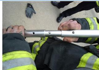
Step 2—To assemble handle, press spring button and insert upper handle into the lower handle until spring button engages.
