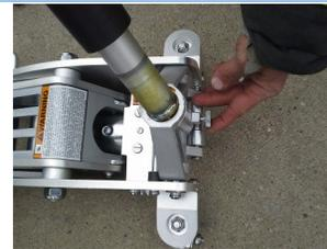
Step 3—Place handle into handle socket on jack and make sure bottom of handle engages the release valve u-joint.
