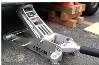
Step 6—Pump handle to lift vehicle using slow and steady pumps until desired height is reached.
