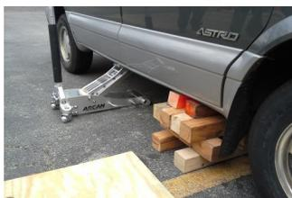
Step 5—To operate jack, turn handle clockwise until it stops. Center saddle plate under load.
