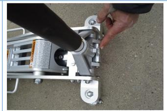
Step 4—Tighten screw to secure handle into the yoke of the jack.
