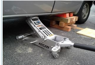
Floor jack in use for lifting operation—note cribbing
