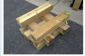
Box cribbing or other load transferring system used with jack at all times.
